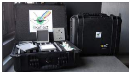
Figure 22 the xDRreflect gloss scale is made of 42 samples.
