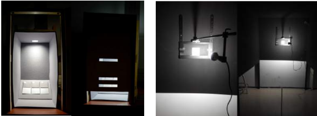
Figure 10 : Light booths for accessing the visual sensation of sparkle. Left, 2 photos of the booths developed by INRIM (with samples on the exhibition plane and with the observation shield). Right, prototype booth developed by UA.
