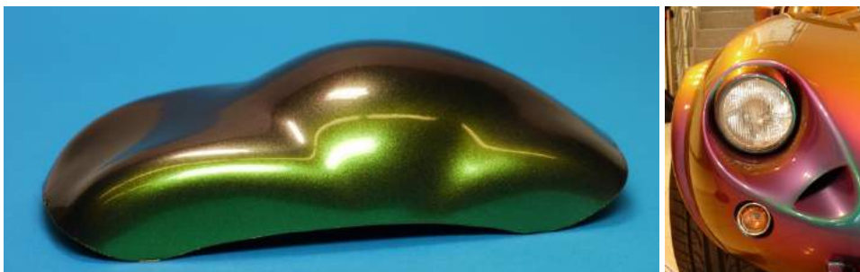
Figure 8 : Examples of goniochromatic coatings. The colour depends upon the direction of illumination and the direction of observation.
