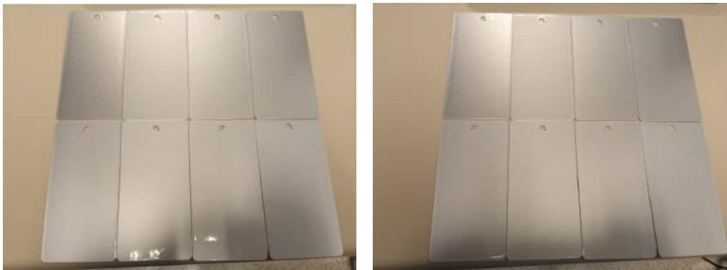
Figure 24 Samples with silverdollar pigment (left) and with cornflake pigments (right)
