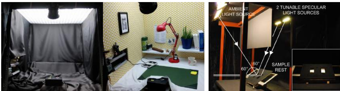
Figure 9 : 2 light booths for accessing the visual sensation of gloss. Left, booth developed by CNAM has 2 possible configurations, “black” or “open space office”. Right, booth developed by KU Leuven.
