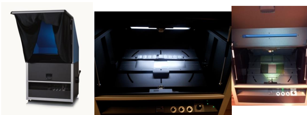
Figure 2. Commercial directional lighting booth using for color evaluation of gonio-apparent colors: byko-spectra effect with some pictures of its interior (center: for color evaluation; right: for sparkle evaluation at 45° geometry).
